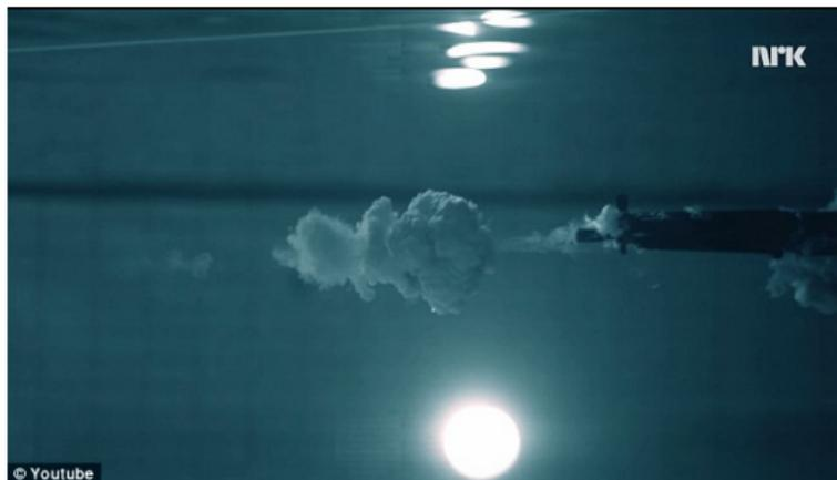
**Figure:** A bullet moving through water has a Reynolds number of around  $10^7$ . The Reynolds number is even higher in air. At such high  $Re$ , the wake of the bullet is extremely turbulent. Source: Andreas Wahl
